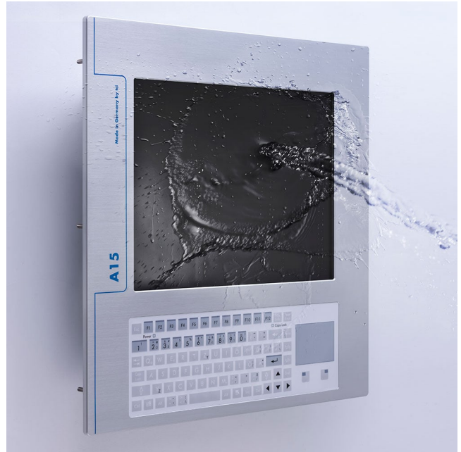
A15-KB front meets the requirements of protection class IP65
